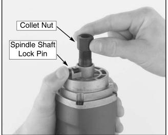
Figure 4. Threading collet nut onto spindle.
